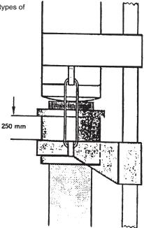
Distance should be at least 250 mm so that pile helmet does not knock against pile helmet holder when pile penctrates fast.
