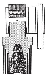
base and the top surface of the insert,when using these together If these surfaces have just slight imperfections,the pile hetmet will crack after just a short period of time.
