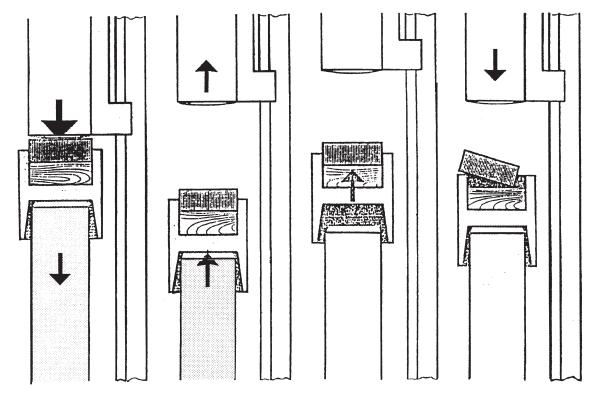
The steel plate is secured either direct to the pile hetmet or via the retaining cables, with which the pile helmet is suspended on the pile hammer and remains connected.during the entire pile driving operation.
