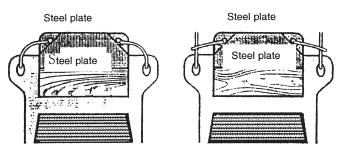
If the steel ptates are cast. it is recommended to cast two eyetets too. Don't weld eyelets. The welding seams would break atter just a short period of time due the extra ordinart impact force. Steel piate Steel ptate
