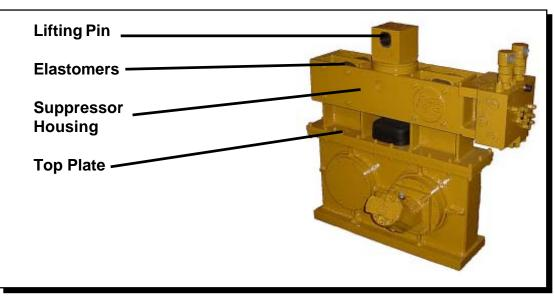
Figure 1-D. General Description of Suppressor Housing.
