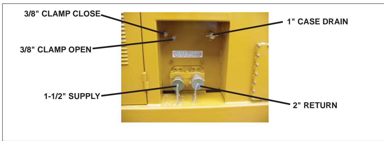
Figure 4-A. Power Unit Coupler Layout
