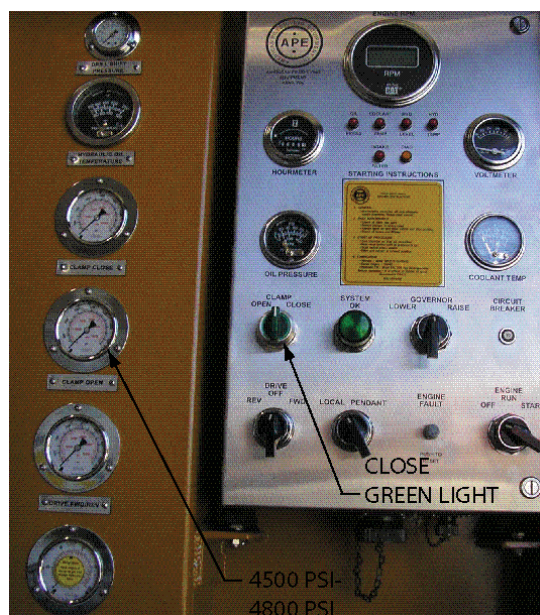
Figure 4-D. Checking Clamp Pressure Switch Setting
