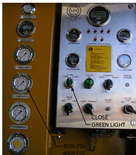
Figure 4-D. Checking Clamp Pressure Switch Setting
