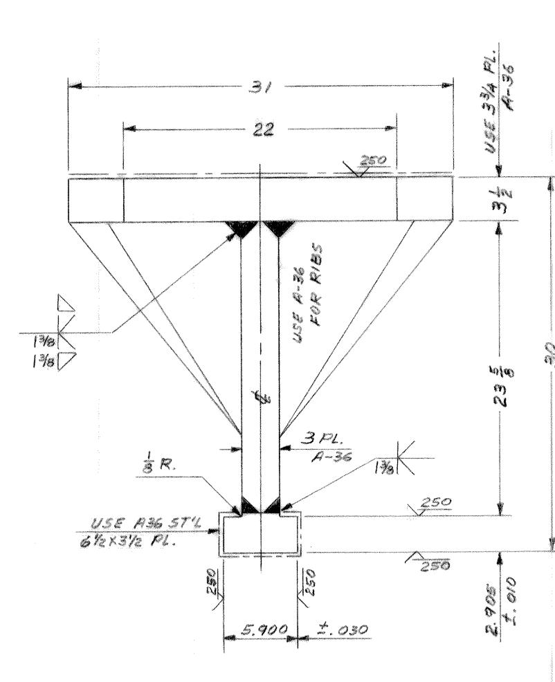
NOTE: 3"WEE PLATE TO BE FLAT WITHIN \$ 1/32 MACHINED FOOT TO BE CENTERED ON 3" WEB PLATE
