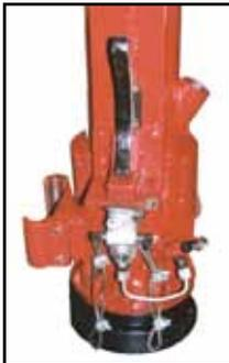
Variable throttle with external pump lever.
