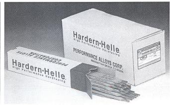
Complex Chrome Carbides with the addition of Boron to add toughness. Develops an even cross checking pattern ideal for severe earth abrasion. Can be applied without shielding gas but use of CO2 will enhance out of position work. Generally limited to 2 layers. 58-60 Rc hardness.
