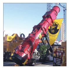
The D180-42 is presently the largest diesel hammer made by Shanghai Engineering Machine Works (SEMW), the APE production facility in China. SEMW is an ISO9002 certified company which purchased the technology from Delmag and has been manufacturing diesel hammers since 1962. Main technical data:
