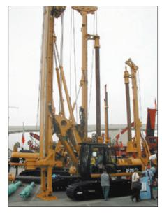
The brand new foundation rig type IMT AF215 is the first of its kind with a telescopic mast. The mast height can be extended from 15700 mm to 25150 mm which allows to make CFA or SDA piles up to 24 m depth and up to 1000 mm diameter. Main technical data:
