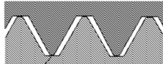
6. IN DRYSEAL (NPTF) THREADS, THE ROOTS AND CRESTS ENGAGE FIRST, ELIMINATING SPIRAL CLEARANCE.
