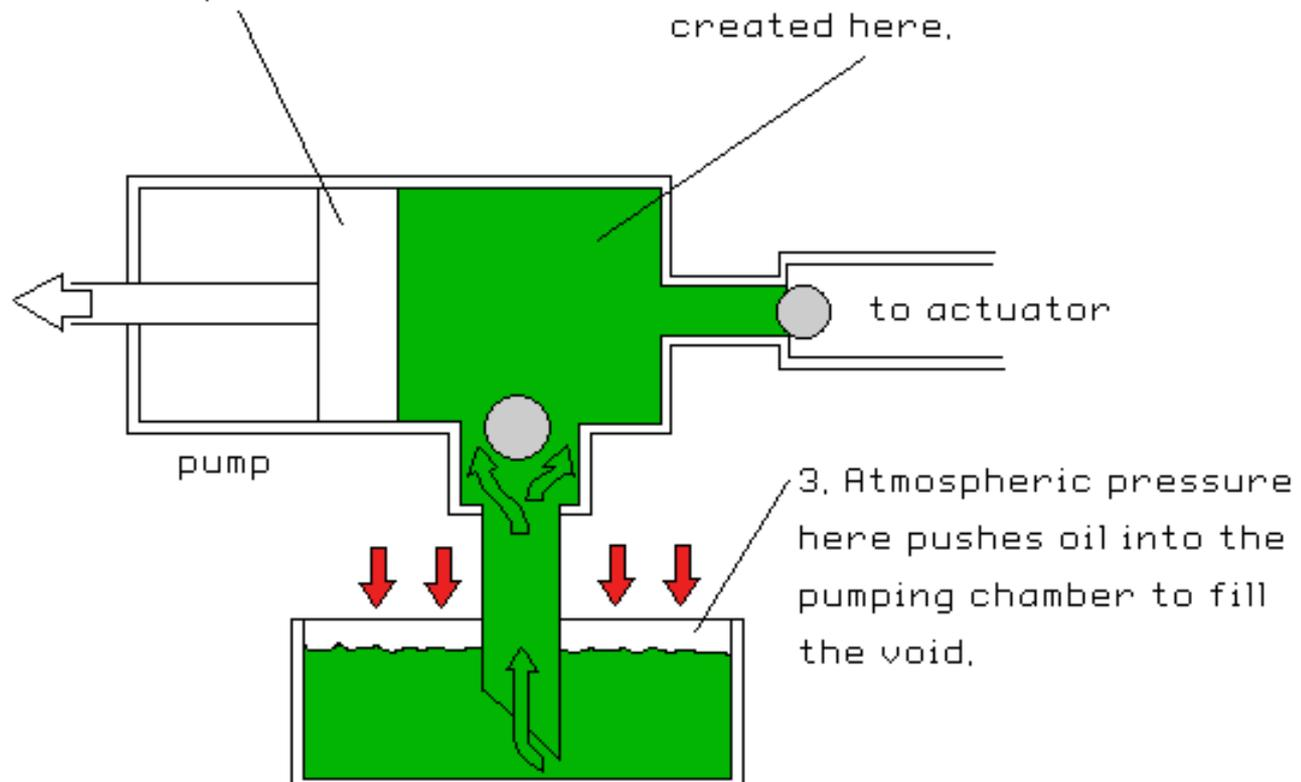
3. Atmospheric pressure here pushes oil into the pumping chamber to fill the void,
