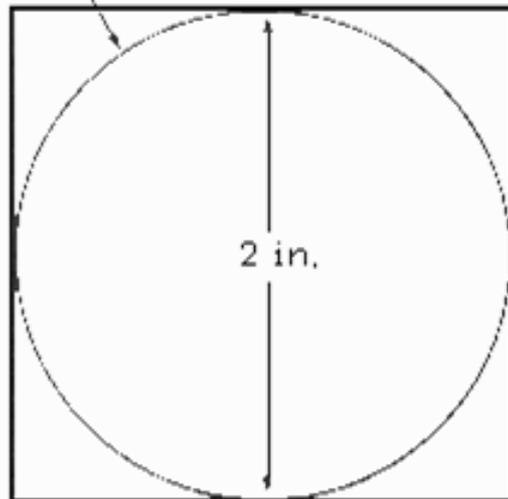
2. It would take four pipes this size to equal the cross-sectional area of the large pipe.
