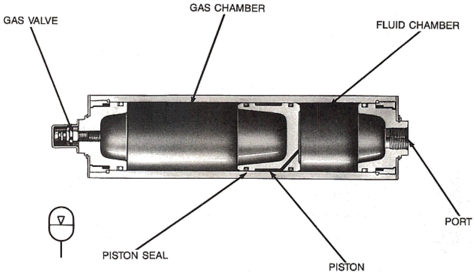
**Figure 18-3. Piston accumulator is gas-charged.**
