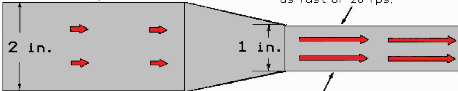
Even if flow in smaller line remains straight, frictional loss will be 16 times more than it is in the larger line.
