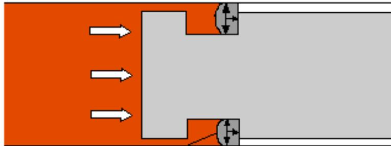
2. WHEN PRESSURE IS APPLIED, THE O-RING IS FORCED AGAINST A THIRD SURFACE CREATING A POSITIVE SEAL.
