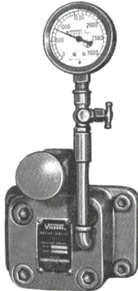
**Figure 18-11. Gauge installed with shutoff valve and snubber.**
