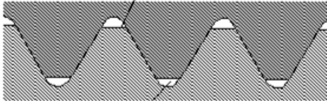
5. THERE CAN BE A SPIRAL CLEARANCE AROUND THE THREADS.
