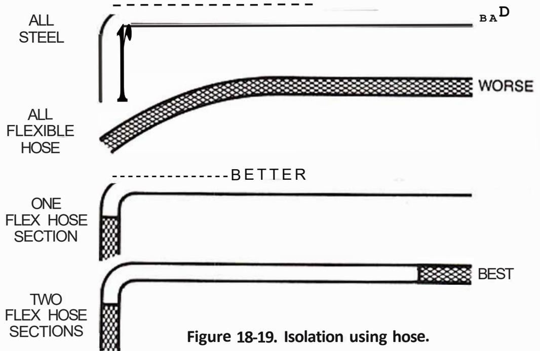
Figure 18-19. Isolation using hose.
