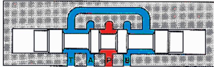
PRESSURED CLOSED—'A' & 'B' OPEN TO TANK
