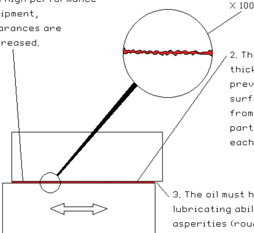
2. The fluid film is not thick enough to prevent the tips of surface imperfections from touching as the parts move against each other,
