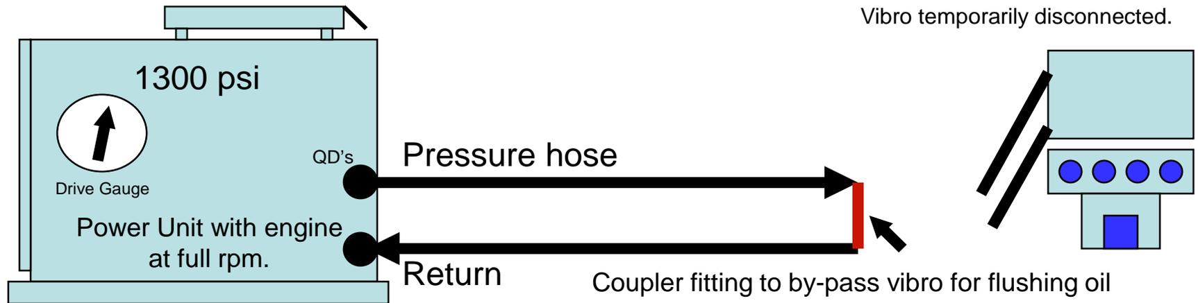
During new production of vibros and drills, we always flush the hose bundle by putting a coupler at the end of the hose bundle. This allows the oil to pass through the drive line hose and go back to the power unit through the return line. We put an in-line filter on the return line to catch the dirt.
