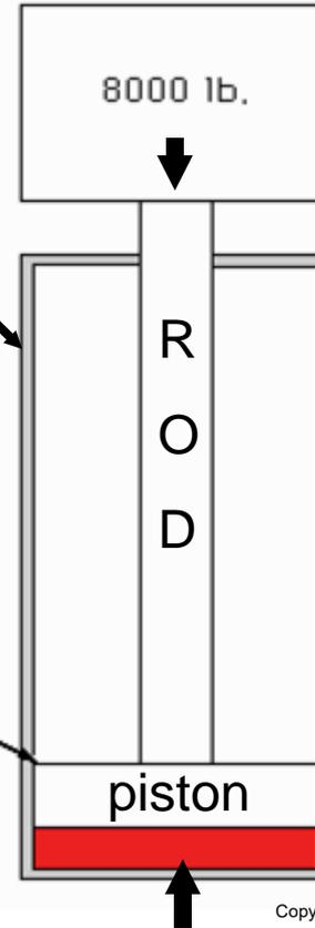
2. the pressure required to lift the load equals the load divided by the piston area:
