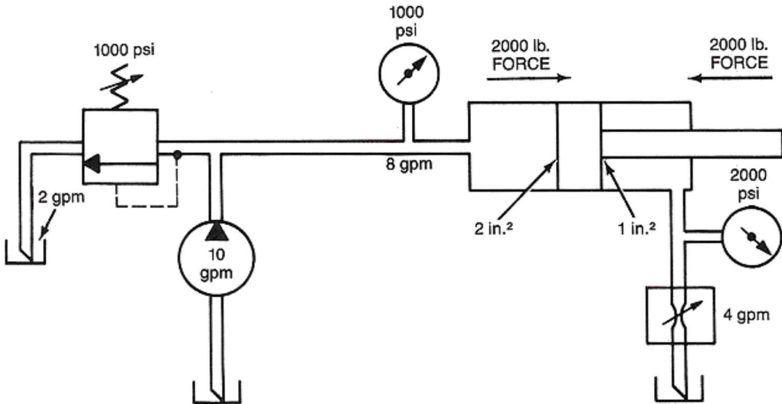
**Pressure Intensification in Meter-Out Circuits**
