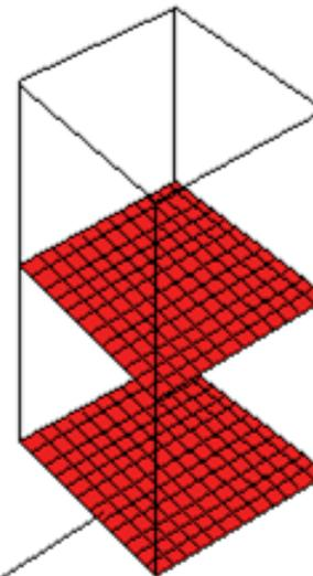
3. A two foot column weighs twice as much, thus the pressure at the bottom is 0.8 psi.
