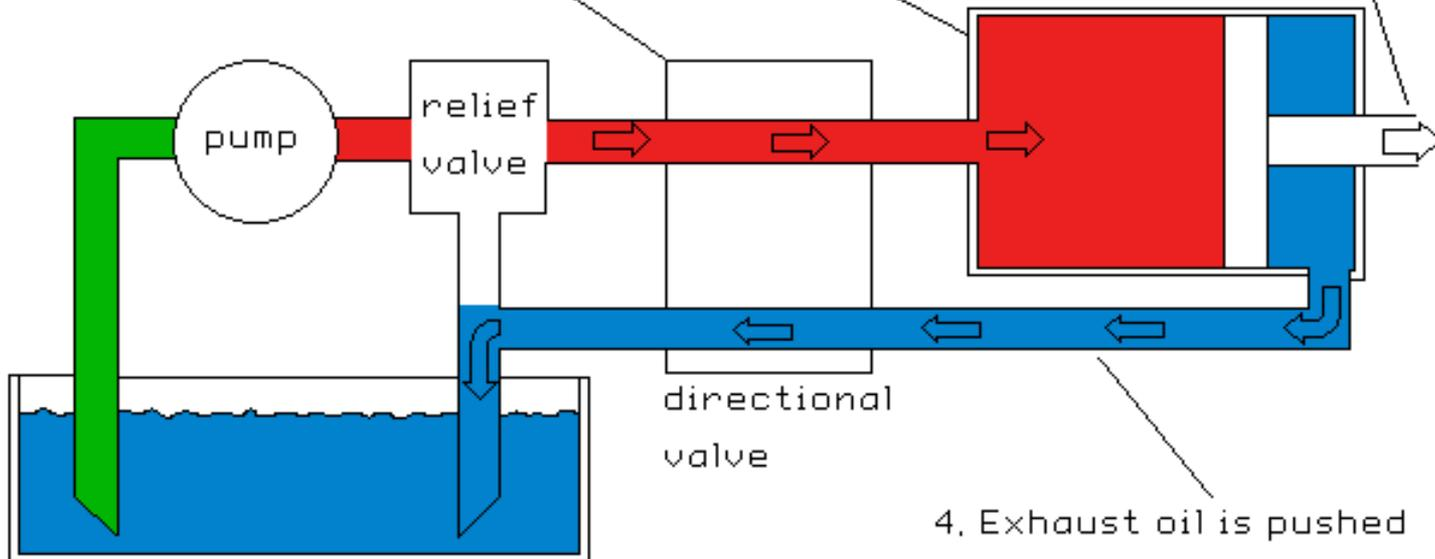
4. Exhaust oil is pushed out of the rod end and directed to the tank.
