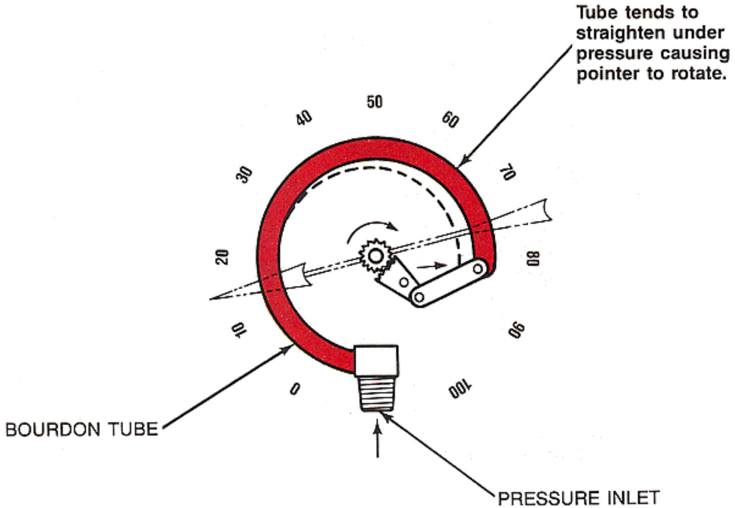
Figure 18-8. The Bourdon Tube gauge.
