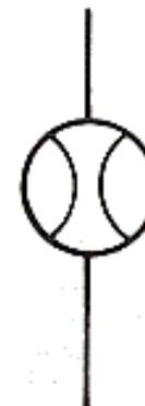
**Figure 18-14. Typical flow meter.**
