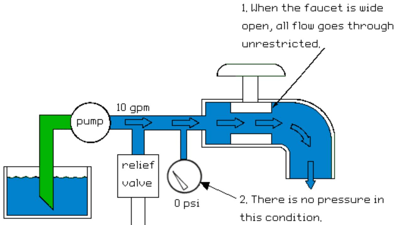
This is like our drive manifold when the vibro is not running. The oil goes through the valve and dumps right back to the tank without building any pressure.
