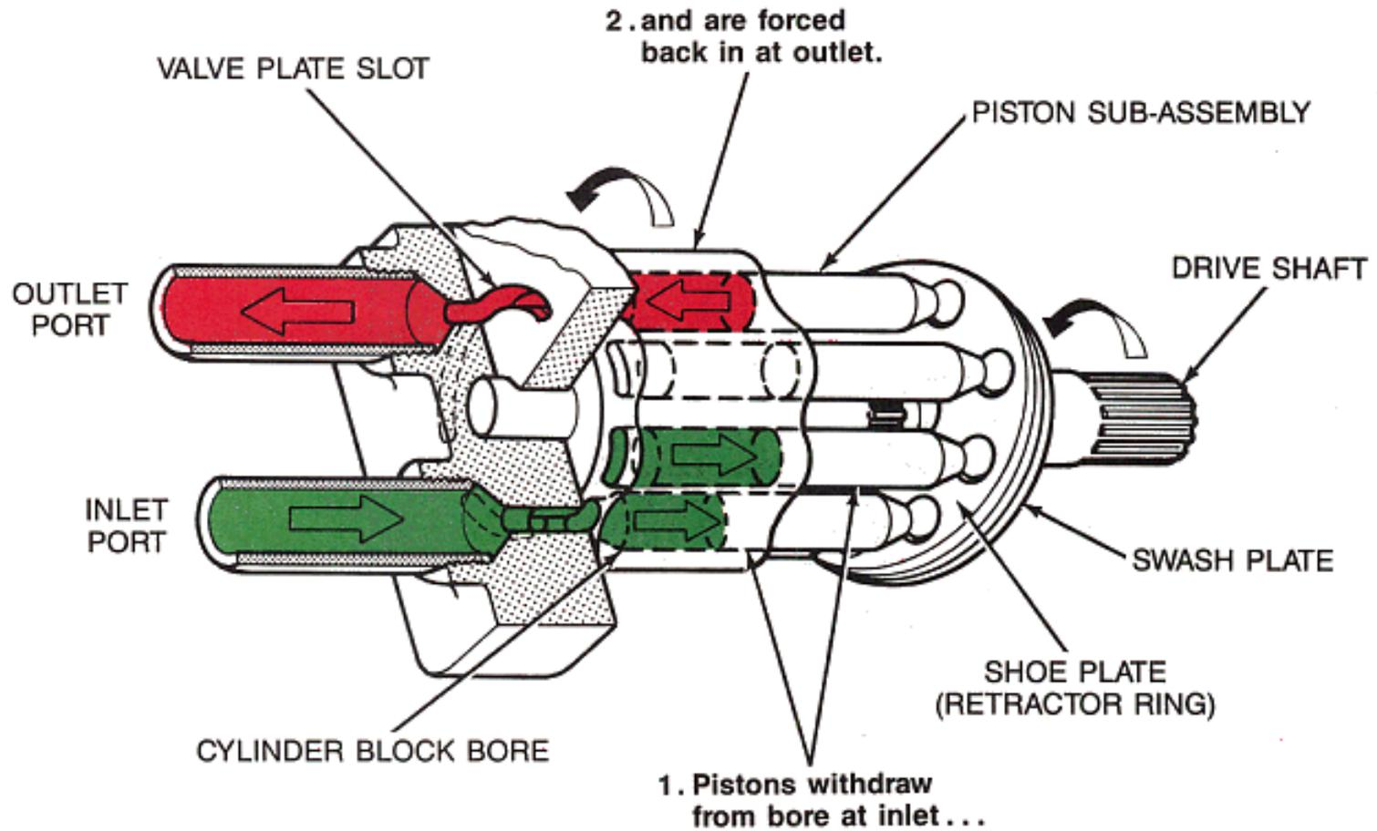
**Figure 17-24. Swash plate causes pistons to reciprocate.**
