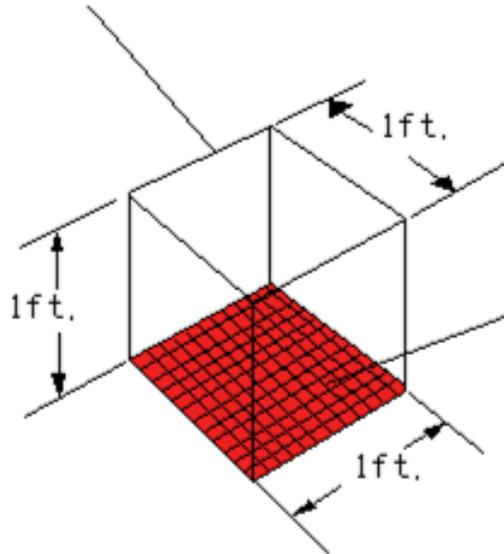
2. If this weight is divided over the 144 sq. in. of bottom, the force on each square inch is 0.4 lb. Thus the pressure at the bottom is 0.4 psi.
