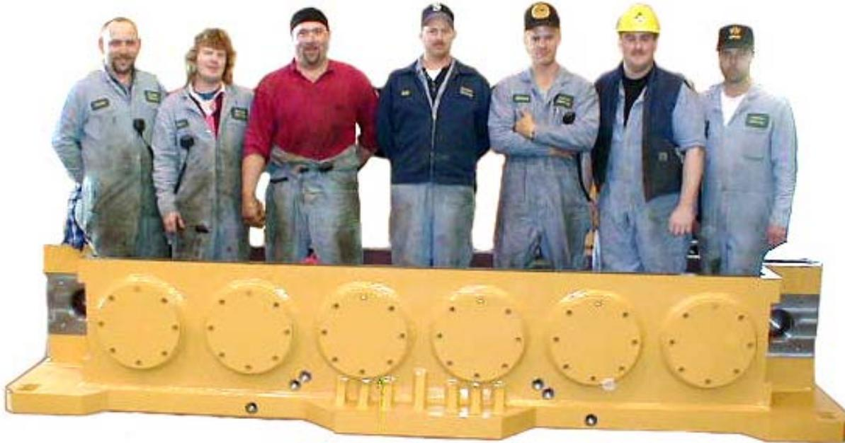
The APE Model 600 is a larger version of the APE Model 400. The 600 has 20,000 inch pounds of eccentric moment. The design is a stretch version of the Model 400. It has six counterweights.
