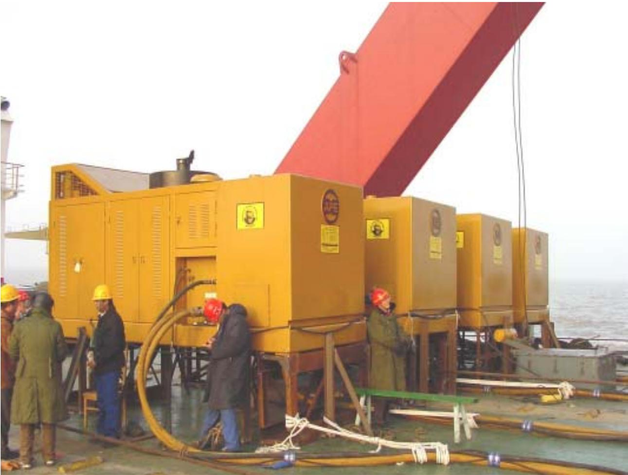
Four APE Model 1000 power units teamed together to provide 4000 horsepower to drive the APE Model 400 Quad Vibratory driver/extractor. Four CAT 3412E electronically controlled engines are fitted to a special control system.
