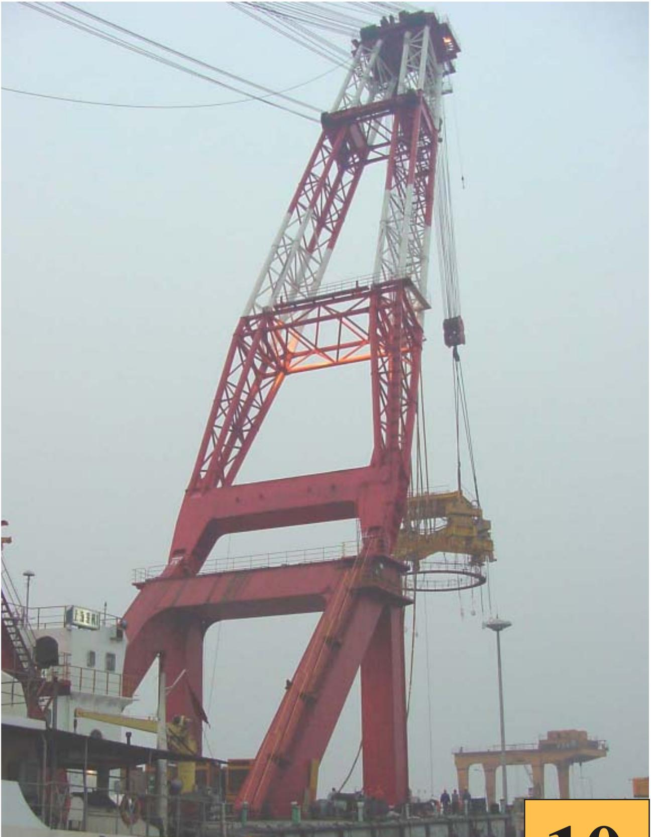
A 1200 ton crane transports the APE Quad Kong down the Yangtze River on its way to the mouth. The APE Quad System is driving two walls of 40 foot diameter concrete piles.
