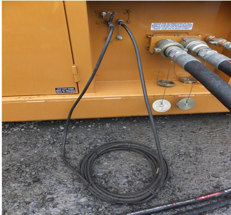
This bulletin is to help with setting the clamp pressure switch. When setting a pressure switch it has to be set in the direction it will be used. The clamp pressure switch changes state when pressure falls to around 4500 P.S.I. from 4800 P.S.I., so we need to set it on the drop.
