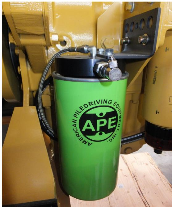
This is the auxiliary engine oil filter kit (1001427) we use in our power units. This unit filters 1 quart per minute at one micron. The inlet is being supplied from the same port as the engine oil pressure gauge. The return oil is set back to a different location on the engine block depending on model.
